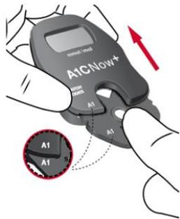
6. "Click" test cartridge into place. Make sure analyser and test cartridge codes must match.
