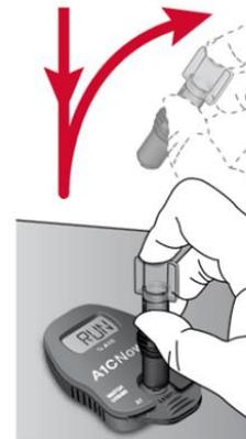
8. Ensure analyser is on level surface. Wait for SMPL to be displayed. Then push down completely to dispense diluted sample. Remove quickly.
