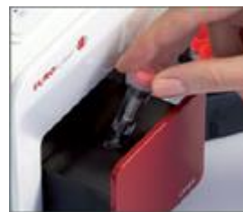
Insert the test cartridge into the instrument
