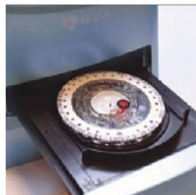
Insert the reagent disc into the analyser
