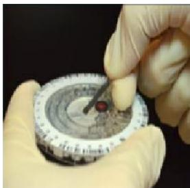
Remove the aluminium strip covering the sample port
