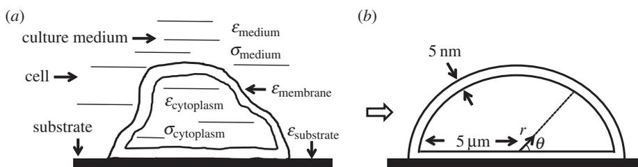
**Figure 3.** (a) Schematic of a cell attached to the substrate. (b) Hemispherical cell model used for simulations. Cell radius is  $5 \mu\text{m}$  and membrane thickness is  $5 \text{ nm}$  (not drawn to scale). Polar coordinate system  $(r, \theta)$  is used to characterize the magnitude of the induced EF in the cell membrane.
