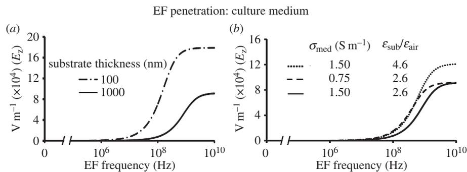
**Figure 8.** Effect of the geometrical and electrical parameters of the stimulation system on  $EF_{\text{induced}}$  in the culture medium. (a) The thinner substrate allows EF penetration into the medium at lower frequencies of the applied field. (b) Decreasing the conductivity of the medium or increasing the permittivity of the substrate shifts the penetration frequency to lower frequencies.
