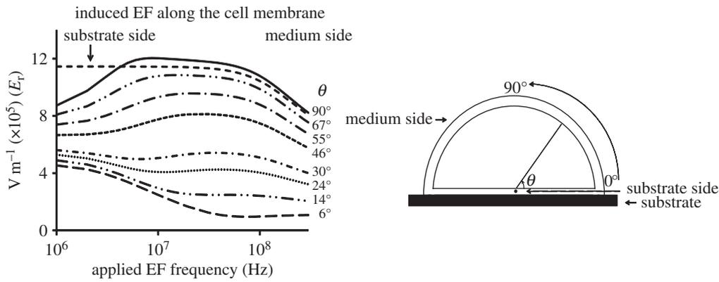
**Figure 6.**  $EF_{\text{induced}}$  as a function of frequency of the applied field at different positions along the cell membrane. Within the  $10^6$ – $10^7$  Hz range,  $EF_{\text{induced}}$  increases near the apex but decreases near the substrate-facing side of the membrane.
