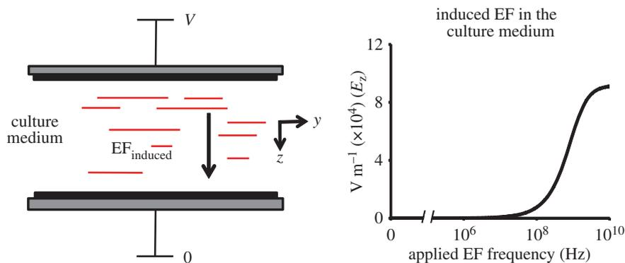
**Figure 2.** Induced electric field in the culture medium as a function of the applied field frequency in the non-contact model. At low frequency of the applied field,  $EF_{\text{induced}}$  is excluded from the culture medium. By contrast,  $EF_{\text{induced}}$  in the culture medium rises dramatically as the frequency approaches 100 MHz and reaches a constant value above 10 GHz. Electrode separation is  $50 \mu\text{m}$  and  $V = 10 \text{ V}$ . (Online version in colour.)
